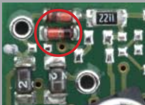
Assembly: e.g. Diode polarity
