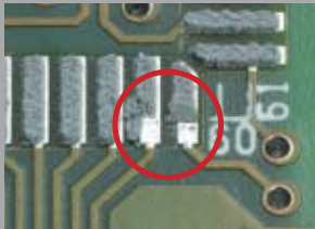
Paste printing: e.g. Smeared paste print
